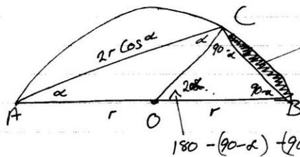
$$\begin{aligned} \text{Shaded} &= \text{Area Sector} - \text{Area } \Delta \\ &= \frac{1}{2} r^2 2\alpha - \frac{1}{2} r^2 \sin 2\alpha \\ &= \frac{1}{2} r^2 [2\alpha - \sin 2\alpha] \end{aligned}$$
